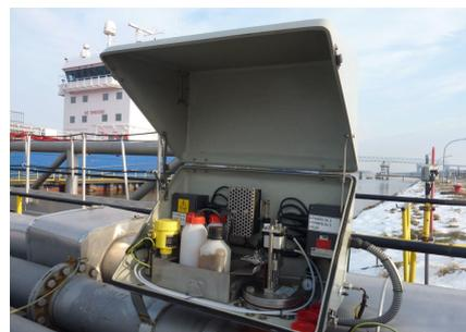
Figure 8 – Automatic MARPOL sampler
