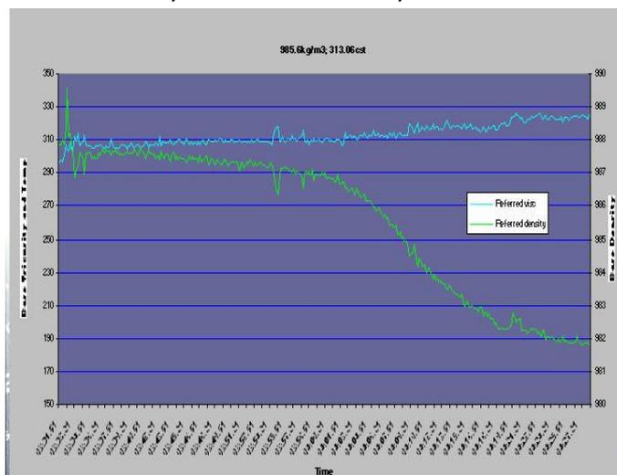
Figure 2 – Layering during tank discharge – source RMI
