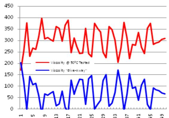
Figure 1 - Viscosity give-away - source Bunkerworld 2009
