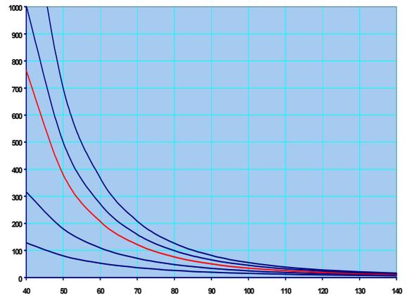
Figure 6 - Heavy fuel oil viscosity/temp index curves
